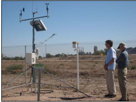
Weather station for irrigation control
